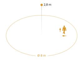
Possible mounting height: 2,00 m - 4,00 m Orange: radial and tangential
